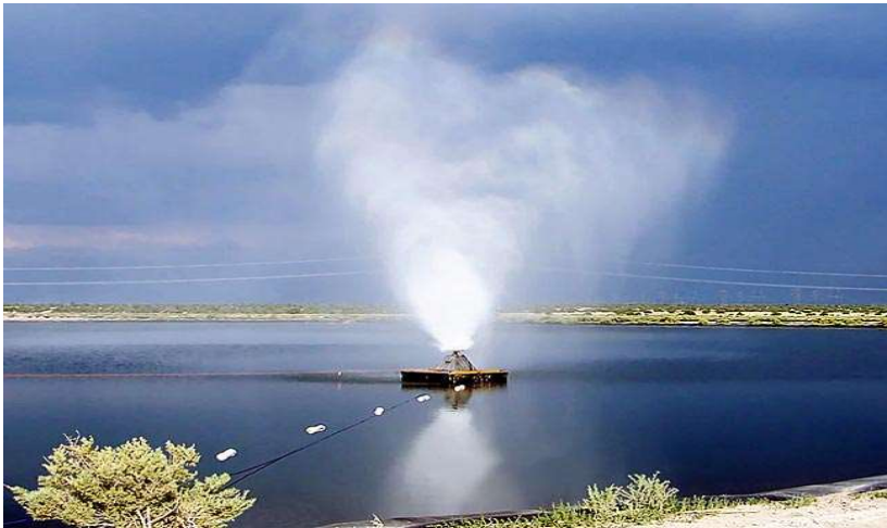
Open evaporation of Leachate in lagoons
